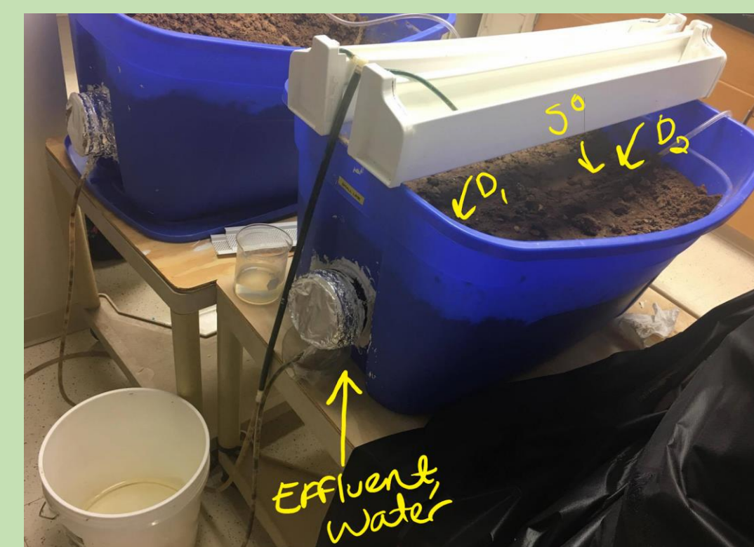
Figure 1: System modeling agricultural drainage. Picture shows sulfur manipulated soil indicating samples taken for DNA extraction: Soil (D1 and D2), sulfur embedded in the draining tubing, and effluent water.
